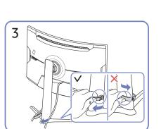
Pull the right side of the HOLDER-STAND CABLE to remove from the stand. The left side of the HOLDER-STAND CABLE can be damaged when pulled forcibly.
