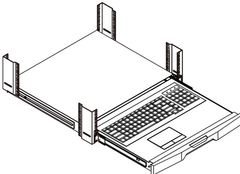
FIGURE 3. INSTALLING THE RM419-R5 KEYBOARD DRAWER INTO THE RACK
