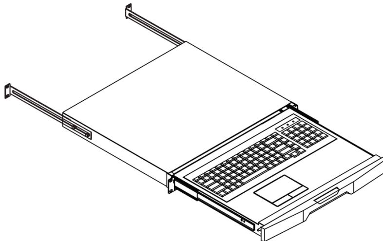
FIGURE 2. ALIGNING THE L-BRACKETS ON THE RM419-R5
