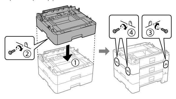
8. Lift up your product and gently lower it onto the paper cassette unit with the corners aligned. Secure the product to the paper cassette unit using the included screws.
