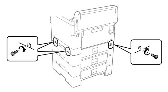
10. Re-insert the protective piece you removed earlier into the back of the lowest paper cassette unit.
