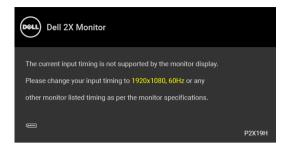
This means that the monitor cannot synchronize with the signal that it is receiving from the computer. See **Monitor specifications** for the Horizontal and Vertical frequency ranges addressable by this monitor. Recommended mode is 1920 x 1080.
