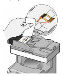
Pull the flap up as shown, and then wipe the sensor behind it.
