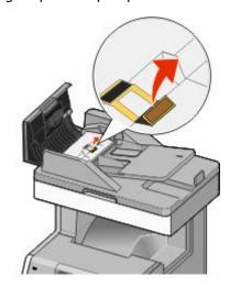
**2** Replace the pick pad with a new one, and then discard the old pad.
