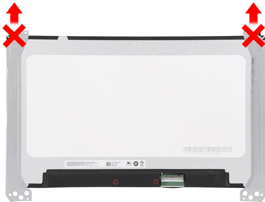
Figure 39. Removing the display panel
