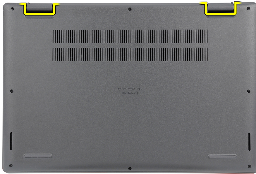
Figure 4. Removing the base cover
