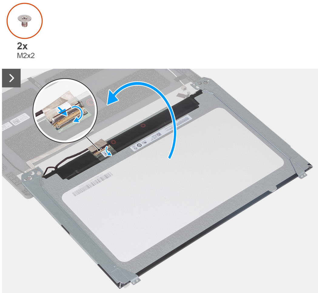
Figure 40. Installing the display panel
