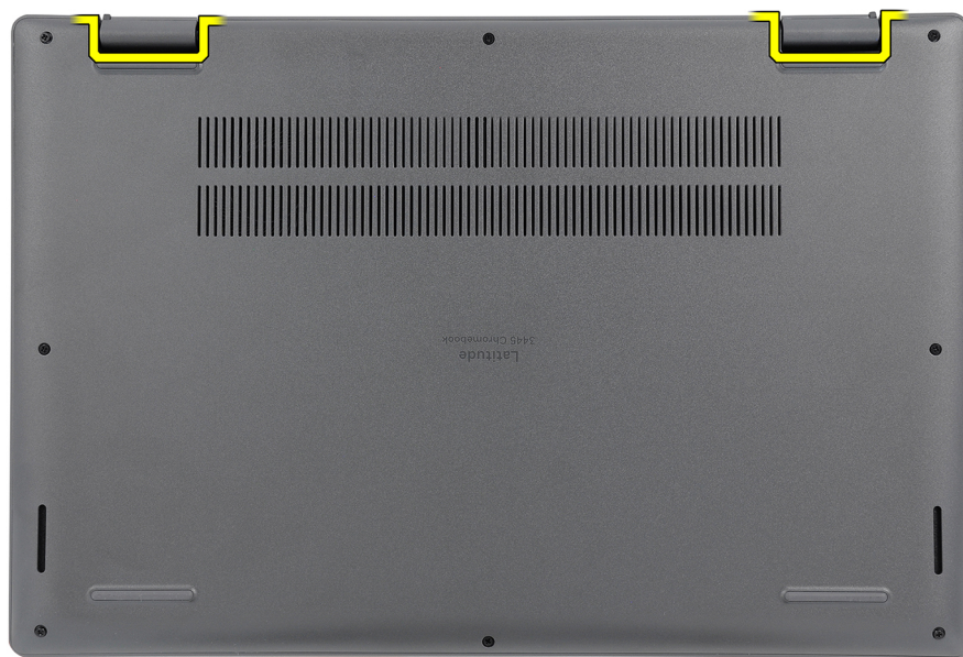
Figure 5. Removing the base cover
