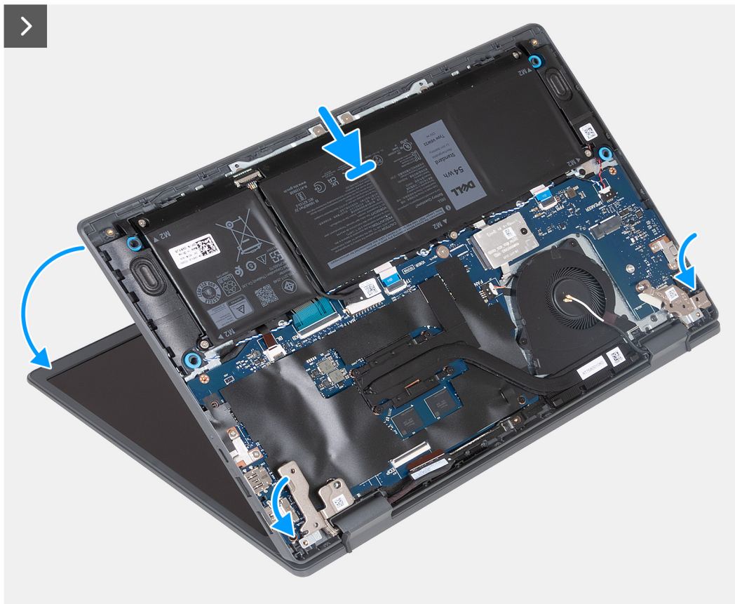
Figure 25. Installing the display assembly
