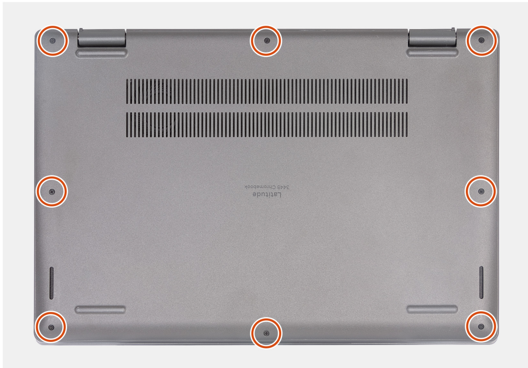
Figure 1. Removing the base cover
