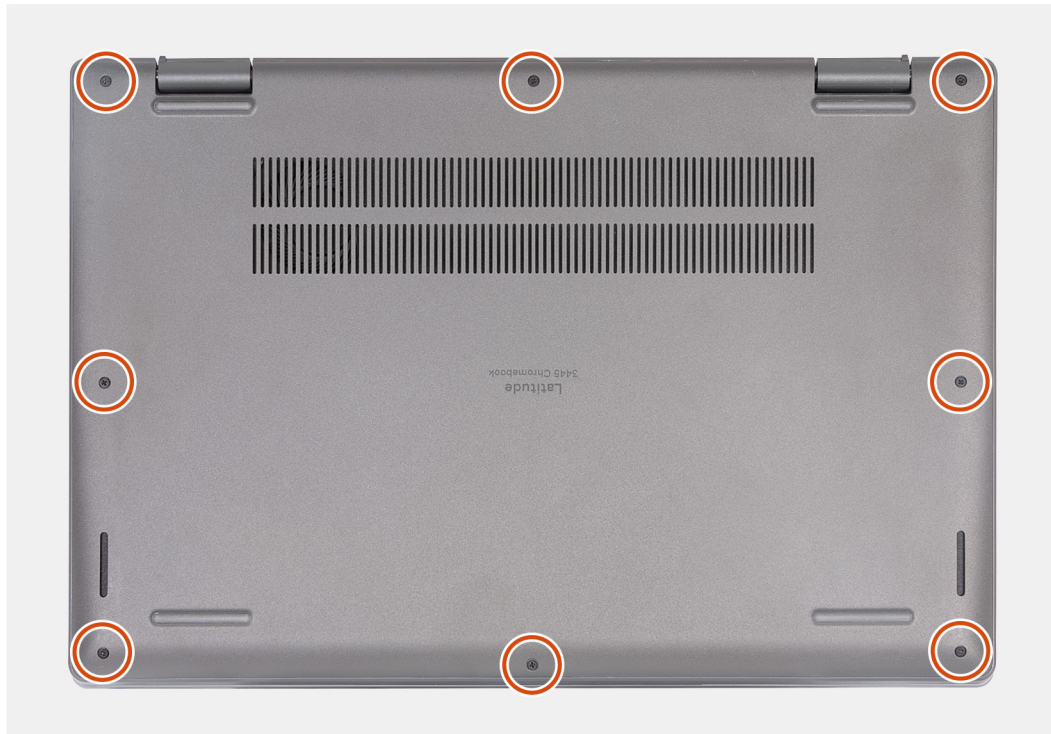
Figure 8. Installing the base cover
