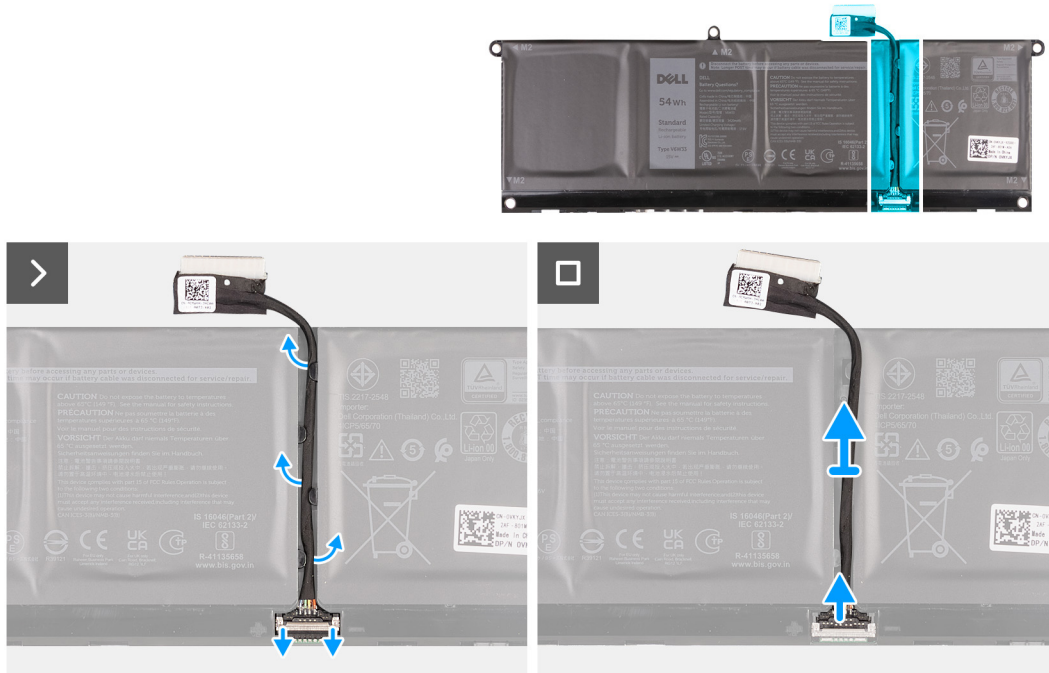
Figure 17. Removing the battery cable
