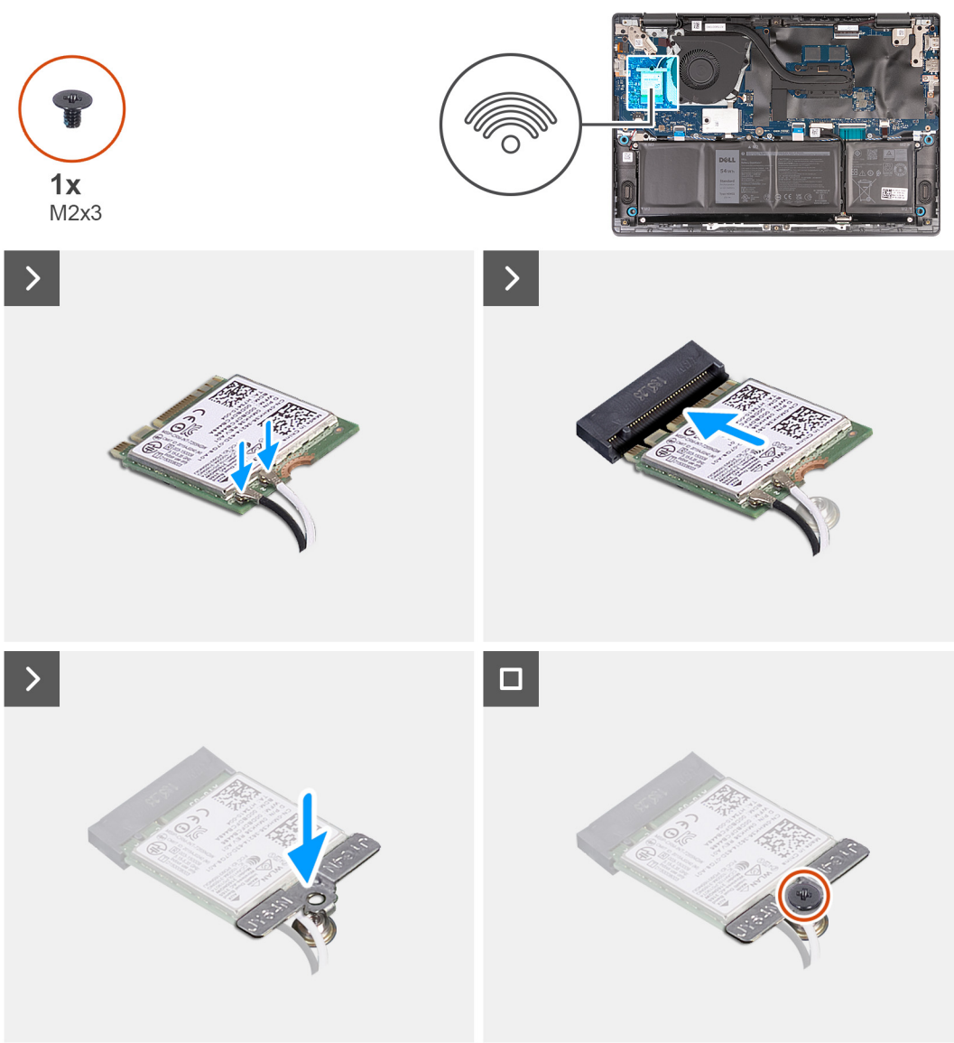
Figure 12. Installing the wireless card
