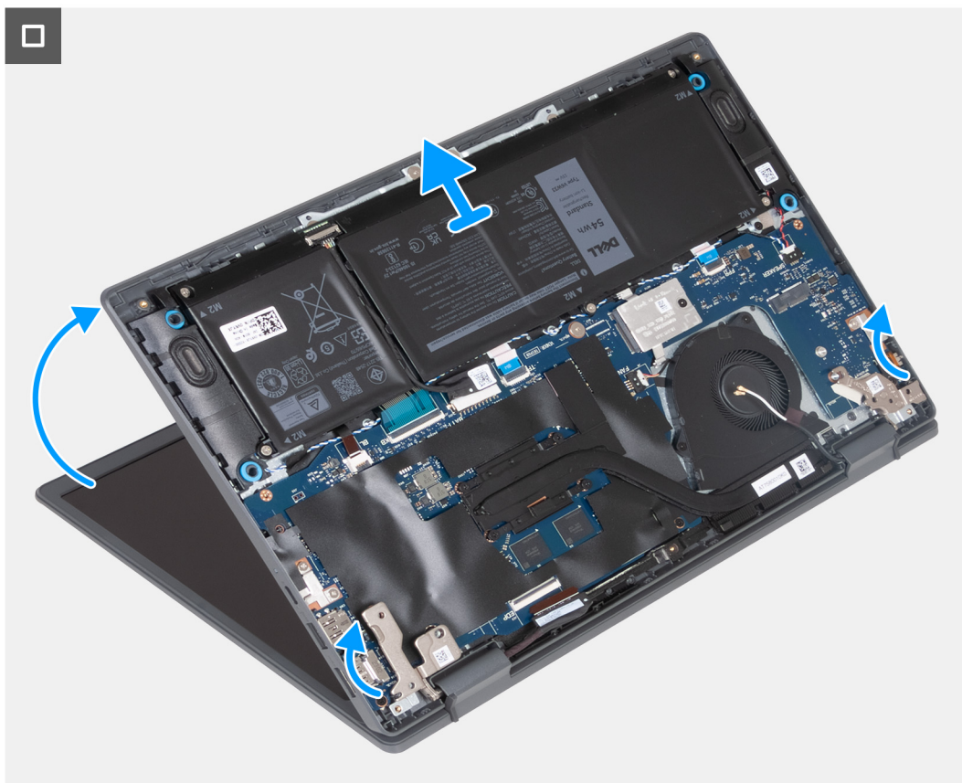
Figure 24. Removing the display assembly
