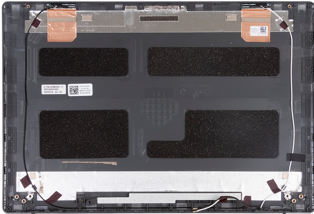
Figure 52. Installing the display back cover and antenna assembly
