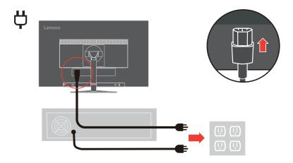
10. Connect the cables with cable clip.
