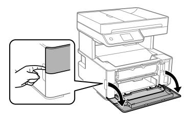
2. Lower the output switch lever.
