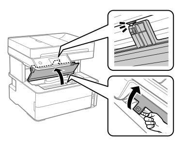
3. Check if the translucent film is smeared. Smears are easier to see if you use a light. If there are smears (such as finger marks or grease) on the translucent film (A), go to the next step.
