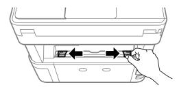
2. Load a single sheet of paper at the center of the rear paper feed slot with the printable side facing up.
