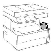
A message is displayed on the printer's control panel prompting you to refill the ink tank to the upper line.
