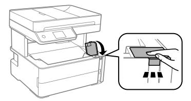
9. Insert the accessory box that came with the printer with the opening flap facing forward as shown below.
