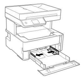
4. With the printable side facing down, load paper until it touches the back of the paper cassette.
