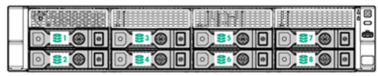
8-bay LFF hot-plug drive model
