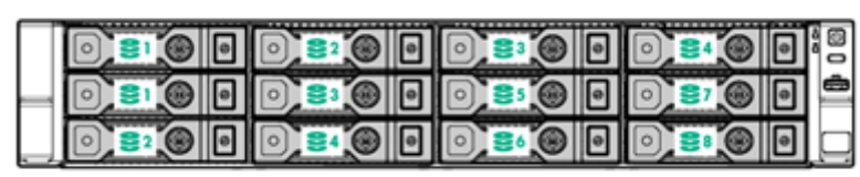
12-bay LFF hot-plug drive model
