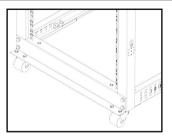
Aligning the Base Bracket with the Vertical Rail
