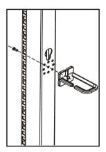
Installing the Cable Management Hooks
