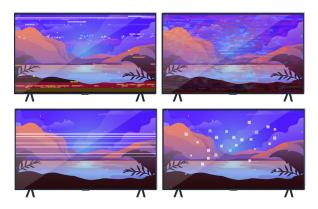
If the issue persists, define exactly what is wrong with the display. For example, mosaics and blocks, multiple lines or white dots, fixed horizontal, or vertical lines.
