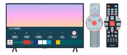
If your TV is connected to the Internet, you can set it to receive periodic updates automatically. On the remote control, press the figure button and move to 🕸 Settings using the directional button.
