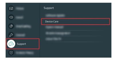
To check sound output, select (a) > (a) Settings > Support > Device Care > Self Diagnosis > Sound Test.
