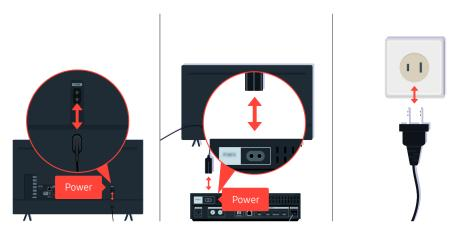
First disconnect and reconnect the power cables and HDMI cables on the back of your TV or the One Connect (OC) Box, then unplug the power cord and plug it back into the wall outlet.
