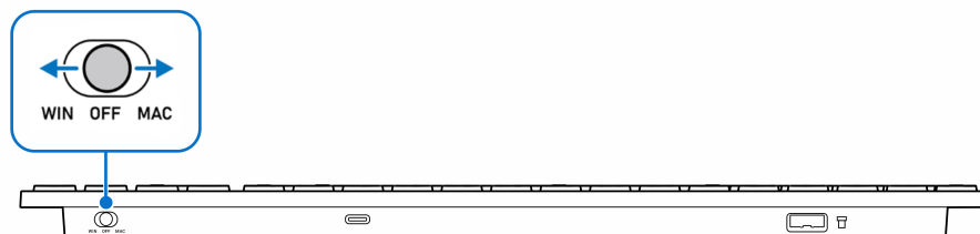
Figure 14. Turning on the keyboard (MAC and Windows)
