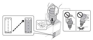
**Note:** Ink flows into the tank and stops automatically when the ink is filled to the upper line. If ink does not flow from the bottle, lift and reinsert the bottle.
