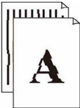
Lines Are Misaligned/Distorted
