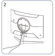
Put both cables in the cable holder on the stand (HOLDER-STAND CABLE) to organize the cables, as shown in the figure. Assembly is complete.
