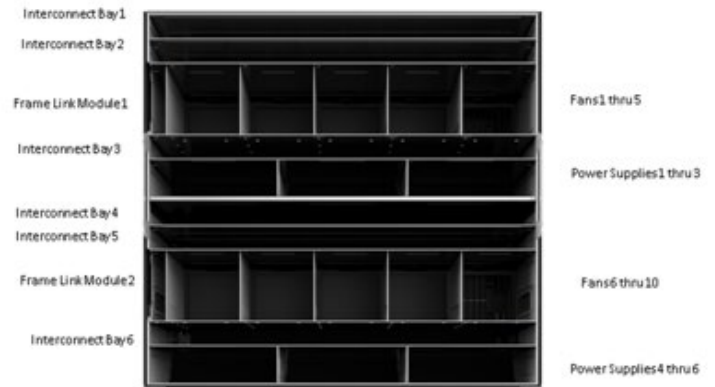
HPE Synergy 12000 Frame - Rear View
