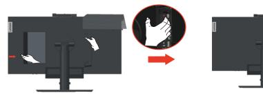
Note: Make sure the Tiny is aligned with the back cover.
