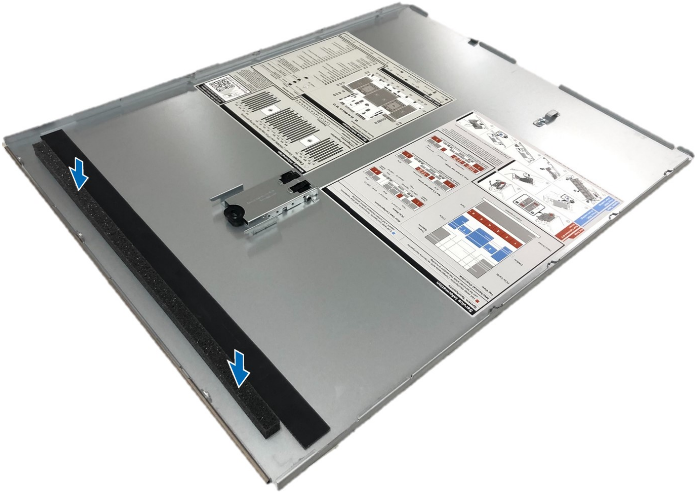
Figure 224. Installing Mylar foam on the system cover
