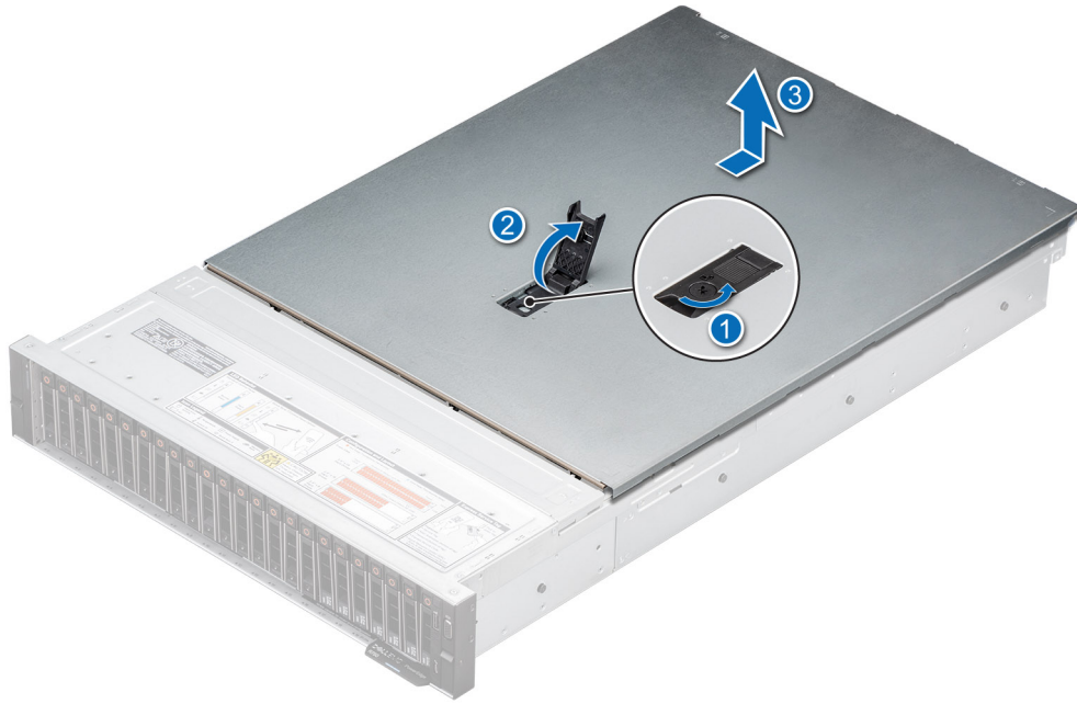
Figure 57. Removing the system cover
