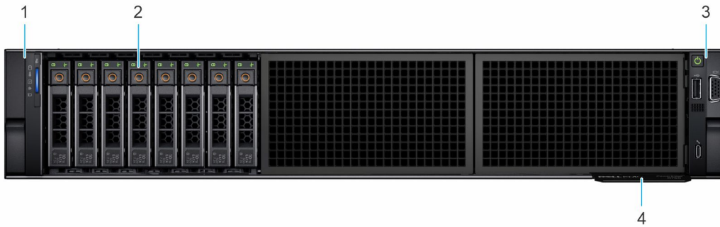
Figure 3. Front view of the 8 x 2.5-inch drive system
