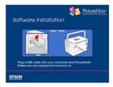
6 Connect the USB cable to any open USB port on your computer. Then connect the other end to the USB port on the back of PictureMate.
