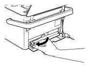
Caution: Do not try to pull out the cartridge without moving the lever.
