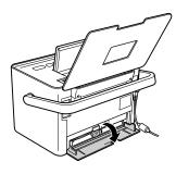
3 Slide the cartridge lever left, to the **Release** position.
