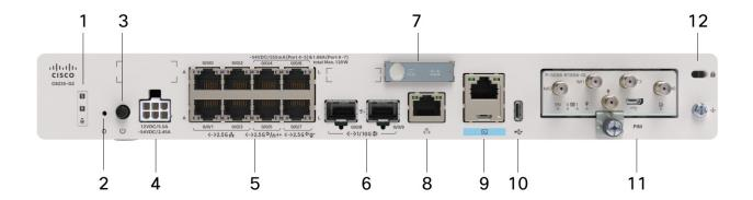
Table 1. Front Panel of Cisco C8235-G2 Secure Router
