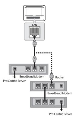
Connect the **LAN** port of the Modem or Router to the **LAN** port on the TV.
