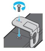
When assembling, make sure the hanger part of the Bracket-Wall Mounts are located behind the rear of the Soundbar.
