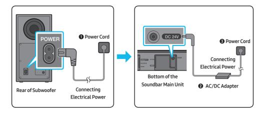
• Make sure to rest the AC/DC Adapter flat on a table or the floor. If you place the AC/DC Adapter so that it is hanging with the AC cord input facing upwards, water or other foreign substances could enter the Adapter and cause the Adapter to malfunction.
