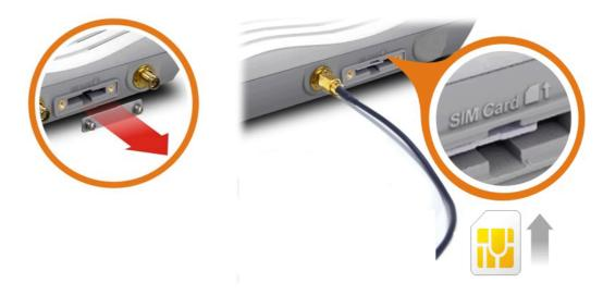
There are two types of antennas provided for Vigor2865Lac, which must be installed in different locations carefully and correctly. Wrong installation might cause bad signal of wireless connection. Therefore, pay attention to the installation of antennas by referring to the following illustration.
