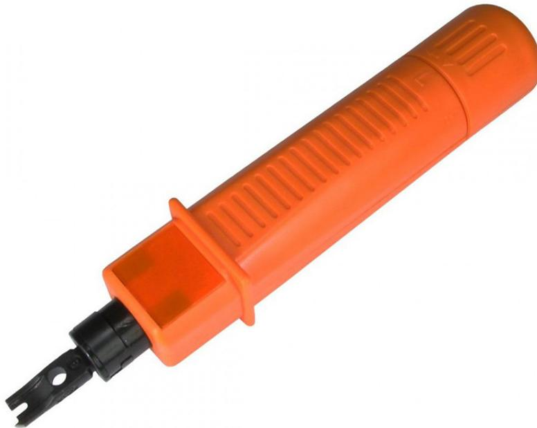
4XEM's professional grade impact punchdown tool is the perfect multi-purpose tool for punching down Cat6a/Cat6/Cat5e/Cat5 cable to 110-Type jacks and patch panels or telephone wire to 66M blocks. Both blades (110 & 66) have cutting and non-cutting sides. Built to perform, this tool features a ridged alloy steel frame with a storage compartment in the body for the blade not in use.
