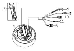
Figure 1-3 Cable Connection of Type II Camera
