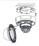
Figure 2-6 Secure the Camera
