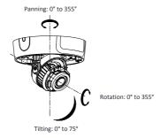
Figure 2-13 Adjust the Angle
