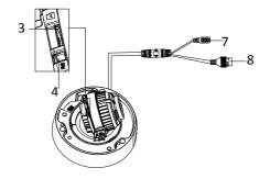
Figure 1-2 Cable Connection of Type I Camera
