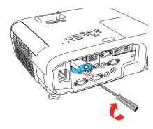
**Note:** The light on the wireless LAN module turns on when the module is installed and operating. The light flashes when the module is communicating over the network.
