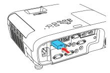
Attach the included wireless LAN module cover and secure it using the screw you removed.
