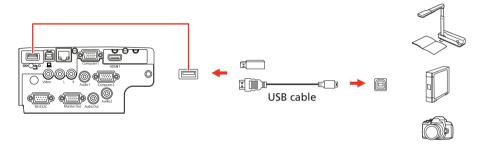
If you connect a digital camera, USB flash drive, or USB storage device, you can use the projector's PC Free feature. See the online *User's Guide* for details.
