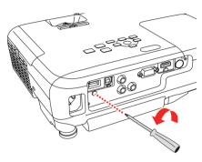
Insert the wireless LAN module into the USB-A port.
