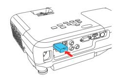
Attach the included wireless LAN module cover and secure it using the 3 screw you removed.
