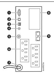
**1** SERIAL COM-serial communication port for:
