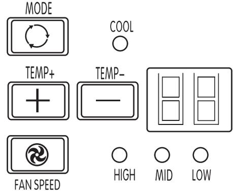
To set the temperature in Cool Mode, press the TEMP+ and TEMP- Buttons. The temperature selected will display in the Display LCD.
