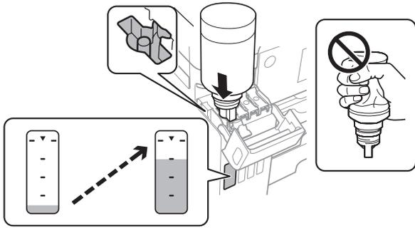
**Note:** If ink does not flow from the bottle, lift and reinsert the bottle.
