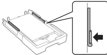
**Note:** Make sure the paper is under the arrow mark on the edge guide.
