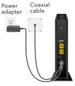
We recommend connecting directly to the cable wall outlet. If you must share the connection, use a 3.5dB (1 to 2) splitter.
