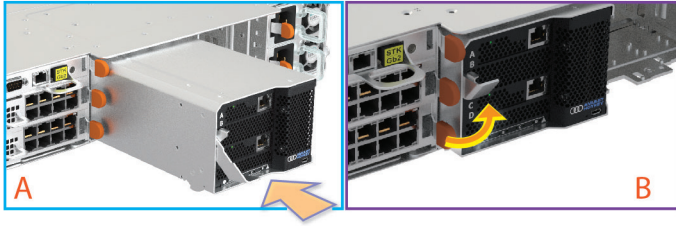
Figure 4: Install the Quad-Expansion module in the Left Hand Side (LHS).
