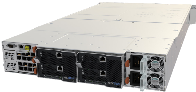
Figure 5: FX2s chassis with two Quad-Expansion modules installed
