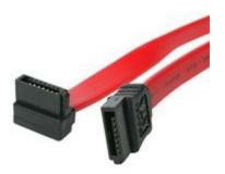
The SATA12RA1 Right Angle (90-degree) SATA Cable features a standard (straight) SATA receptacle as well as a right-angled SATA receptacle, providing a simple 12-inch connection to a Serial ATA drive, with full SATA 3.0 bandwidth support of up to 6Gpbs when used with SATA 3.0 compliant drives.
