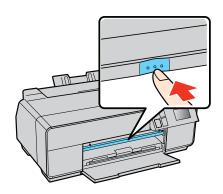
Insert a single sheet of fine art media. Insert it short end first with the printable side faceup.
