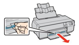
3 Load paper against the right edge and behind the tab. Then press the button on the edge guide and slide it to the edge of the paper.
