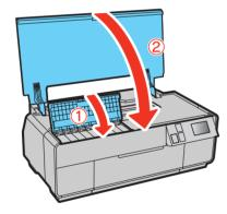
The printer begins priming the ink delivery system. This takes about 10 minutes. Do not turn off the printer, load paper, or open any covers until the process is complete.
