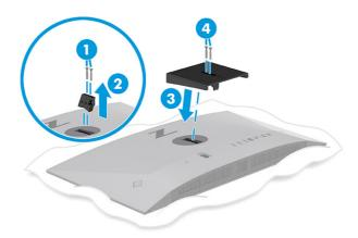
2. Remove the four screws from the VESA holes located on the rear of the monitor head.
