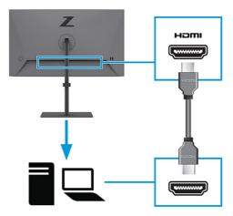
• Connect one end of an HDMI cable to the HDMI port on the rear of the monitor and the other end to the HDMI port on the source device (camera model).
