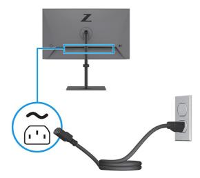
Connect one end of the power cord to a grounded AC outlet. Then connect the AC adapter to the power connector on the monitor (camera model).
