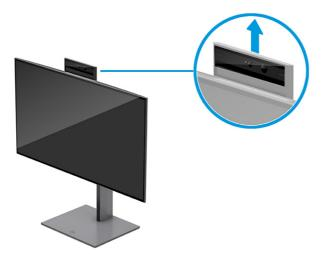
NOTE: If a camera firmware update is required, unlock the camera before updating the firmware.
