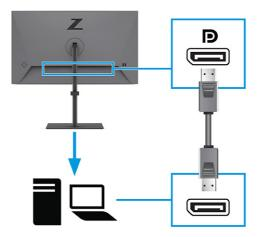
• Connect one end of a DisplayPort cable to the DisplayPort connector on the rear of the monitor and the other end to the DisplayPort connector on the source device (camera model).
