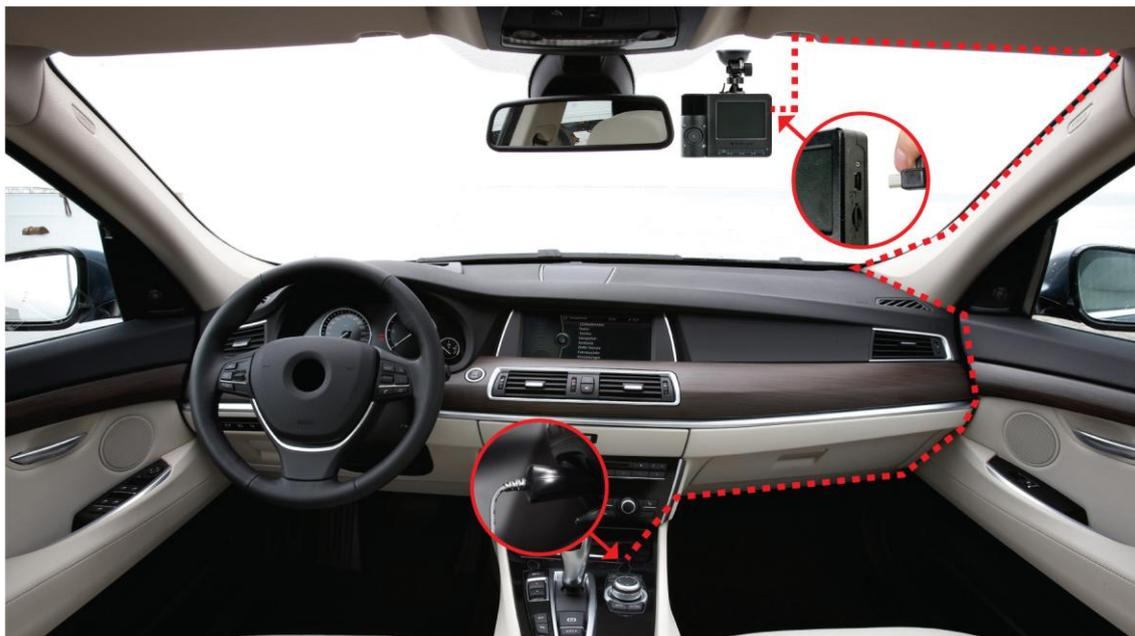
1. Connect the micro USB cable to the DrivePro.
