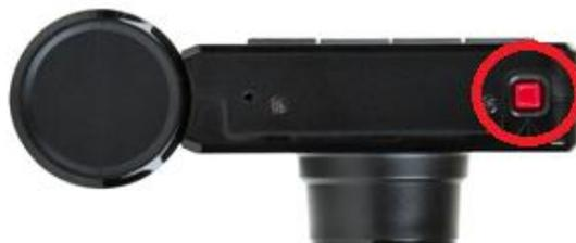
A warning will appear on the screen when the emergency recording is being activated.
