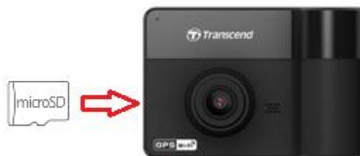
**Note:** Always format new memory cards in the DrivePro before using them for the first time. To format a new memory card, press the Settings button during recording, and select **Format Card**.
