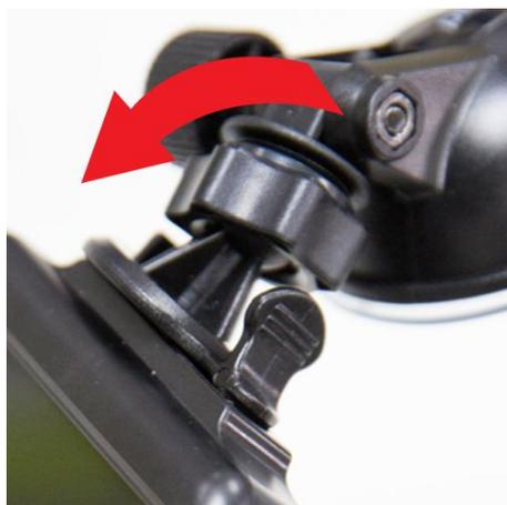
5. After the DrivePro is in the best position, turn the adjustment knob clockwise to make sure that the DrivePro is securely locked in place.
