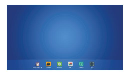
Switch to Embd Player source to display main interface as show above. Press LEFT/ RIGHT key on remote control to select icon below, and press Enter key to enter corresponding program, or click icon directly with touching pen to enter program. In any program, to press Home key on front panel of display to return to the main interface.
