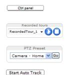
Click the Ctrl panel button to open the PTZ control panel which provides additional PTZ controls. User-defined buttons can also appear in the Control panel. See *Controls on page 31*.
