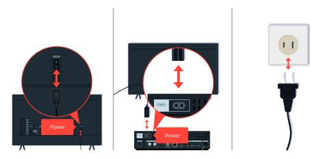
First disconnect and reconnect the power cables and HDMI cables on the back of your TV or the One Connect Box, then unplug the power cord and plug it back into the wall outlet.
