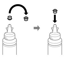
Close the cap onto the ink tank securely.
