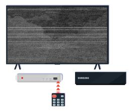
If you use an Multi-Brand Remote (MBR) or universal remote and your remote cannot operate an external device, move the external device closer to the One Connect Box.
