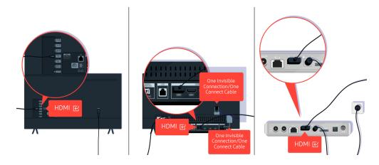
Check the connection of the HDMI cable to your TV or One Connect Box.
