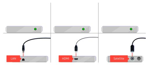
If you are using a set-top box, check the cable connection. The cable you need to check depends on the type of set-top box.
