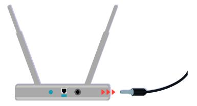
Try rebooting the access point by disconnecting and reconnecting the power connector. It may take 1 to 2 minutes until the access point comes back online after a reboot.
