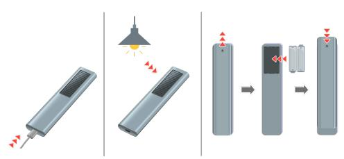
If you cannot see infrared signals, charge the remote control by using the USB port (C-type) on the bottom, or turn over the remote to expose the solar cell. If the remote control has batteries, replace them with new ones.
