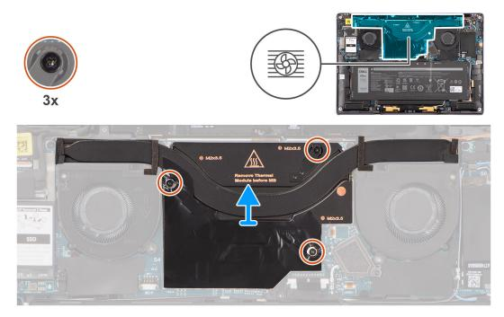
(i) NOTE: To remove the heatsink shielding cover, pry it open from the recess located at its top right corner.
