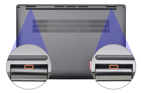
3. Pry open the base cover from the top, left, and right sides of the base cover.
