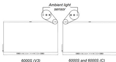
On SMART Board 6000S (V3) models, the ambient light sensor is located in the top-right corner of the display's frame. On the 6000S and 6000S (C) models, the sensor is in the top-left corner.
