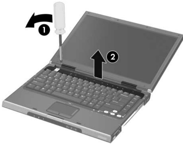
Releasing the Switch Cover, HP Pavilion dv1000 Notebook Models Only
