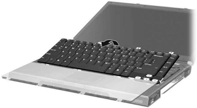
Releasing the Keyboard, HP Pavilion dv1000 Notebook Models Only
