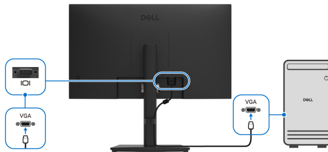
Figure 14. Connecting the VGA cable
