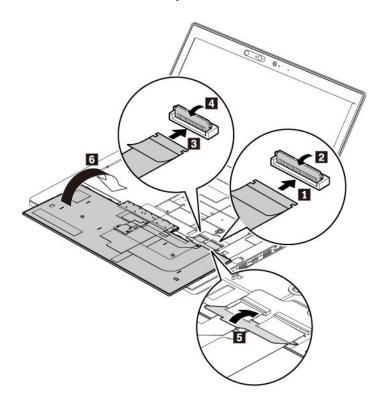
2. Insert the keyboard into the keyboard bezel as shown. Ensure that the top edge of the keyboard (the edge that is close to the computer display) is under the frame of the keyboard bezel.
