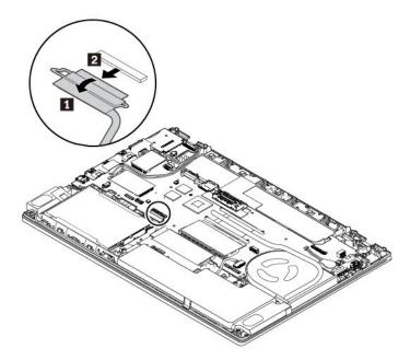
7. Pull the tape to remove the M.2 solid-state-drive converter and its bracket.
