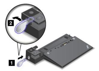
2. Attach your computer to the docking station as shown until you hear a click 1. Turn the system lock key to the locked position (vertical) 2.
