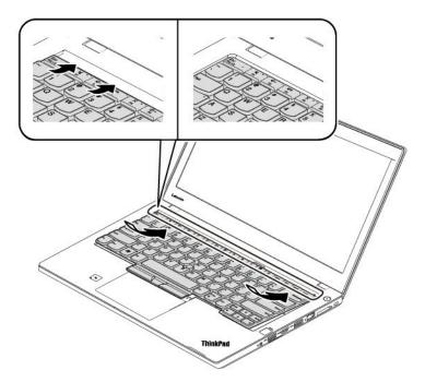
3. Slide the keyboard in the direction as shown by the arrows. Ensure that the latches are secured under the keyboard frame.
