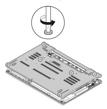
6. Remove the base cover assembly in the numeric order as shown.
