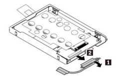
9. Remove the two screws that secure the M.2 solid-state-drive adapter 1, and then remove the adapter 2.
