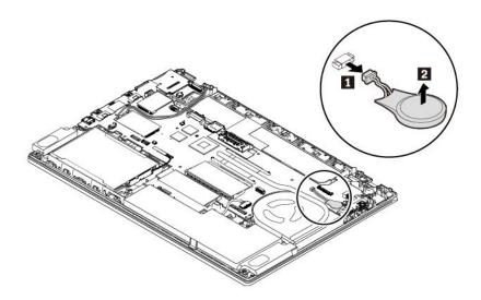
7. Install the new coin-cell battery 1 and attach the connector 2.
