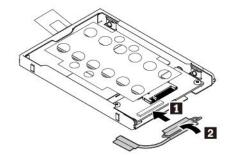
5. Insert the converter 1 and then pivot it downward 2. Ensure that the converter is seated in place and the tape does not cover the speaker.
