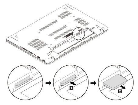
5. Note the orientation of the new micro SIM card and then insert it into the slot completely until it clicks into position.
