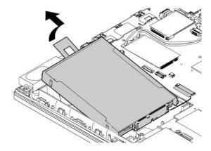
8. Disconnect the cable from the 2.5-inch storage drive.
