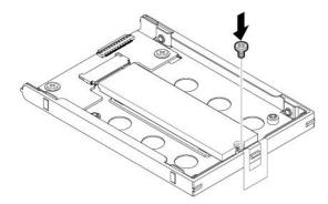
3. Install the M.2 solid-state-drive adapter and then install the two screws to secure the M.2 solid-state-drive adapter.
