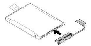
3. Insert the new storage drive 1 and then pivot it downward 2. Ensure that the new storage drive is seated in place and the tape does not cover the speaker.
