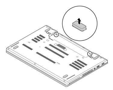
7. Turn the computer over and open the display. Push hard in the direction as shown to release the latches from the keyboard bezel.
