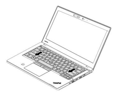
4. Close the computer display and turn the computer over. Lock the keyboard frame.
