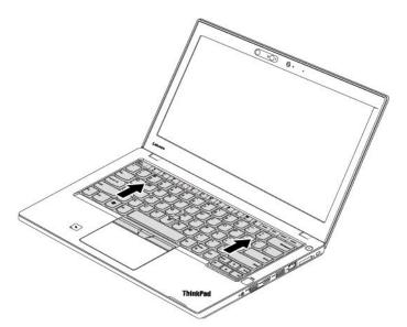
8. Pivot the keyboard slightly upward as shown by arrow 1. Then turn over the keyboard as shown by arrow 2.
