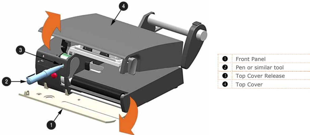
4. Using a Cotton Swab moistened, not soaked, with isopropyl alcohol gently wipe away any build-up on the Printhead surface, paying close attention to the burn line. Allow the Printhead to dry.
