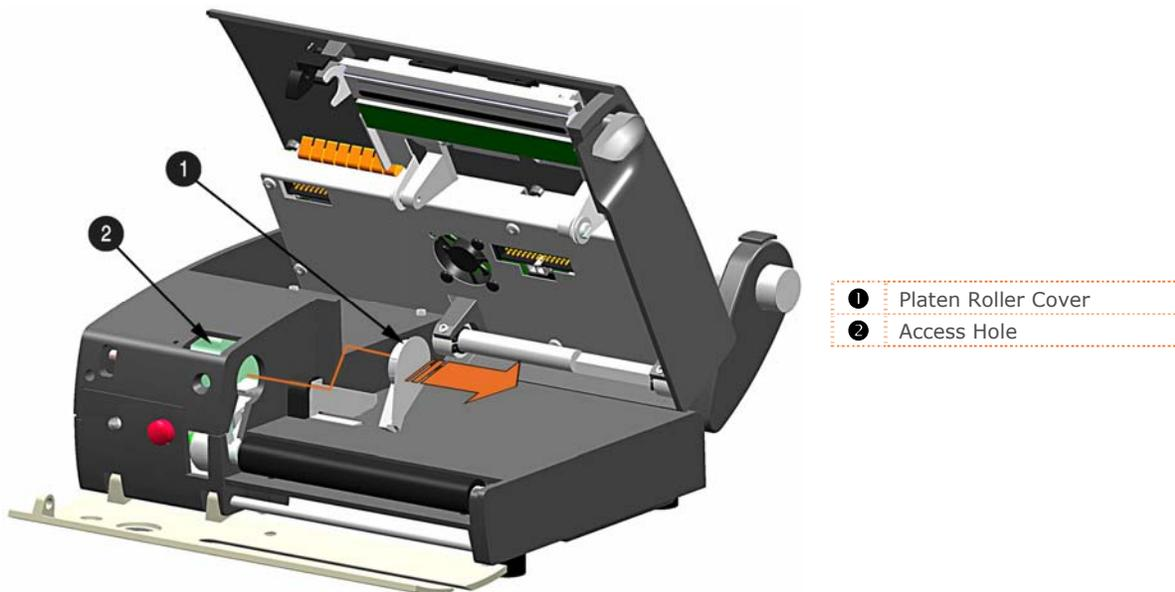
5. Lift the Platen Roller Assembly up and out of the printer
