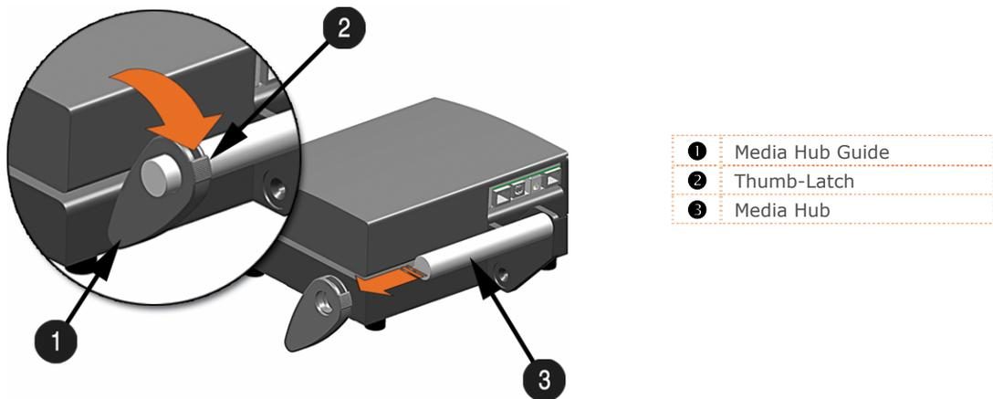
*DC Models:* Loosen the Media Guide Handle and slide the Media Hub Guide off the Media Hub.
