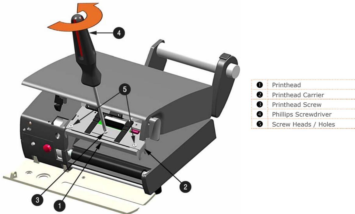
4. It is now recommended to clean the Printhead to remove any oil or dirt from handling. Perform the Printhead Cleaning procedure, (see section 4.2).
