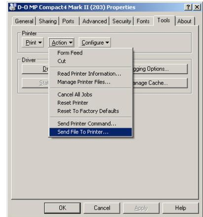
8. As the new firmware is sent to the printer the Status Light will flash as the data is received.
