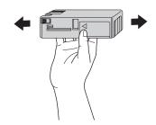
8. Hold the ink cartridge with the arrow mark facing up and pointing to the back of the printer, and then insert it into the slot until it clicks.
