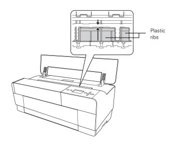
If the problem still occurs, clean the area using a soft, lint-free, dampened cloth. Then wipe the inside of the printer dry with a dry, lint-free, soft cloth.
