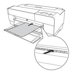
5. Position the right edge of the paper against the right side of the tray and align the paper's bottom edge with the white line on the tray.
