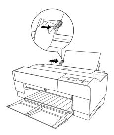
6. Gently guide the paper into the slot until it meets resistance. Maintain a constant pressure; after a few seconds you'll feel the printer pull the paper into printing position.
