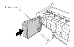
The printer has a protection system to prevent improper cartridge insertion. If you cannot insert the ink cartridge easily or if you see the message INK CARTRIDGE ERROR on the LCD panel, the type of cartridge may be incorrect. Check the package and product code.
