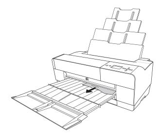
If necessary, open the top cover, and remove any jammed paper from the area shown below.
