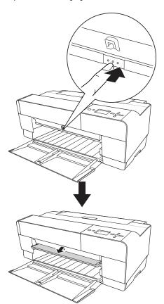
4. Insert a single sheet of paper, short edge first and face-up into the front tray.
