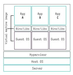
With containers, virtualization is achieved at the operating system [OS] level instead of at the hardware level like virtual machines.
