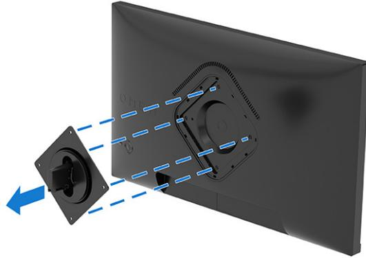
3. To attach the monitor head to a swing arm or other mounting device, align the mounting plate on the swing arm with the screw holes on the back of the monitor head (1).
