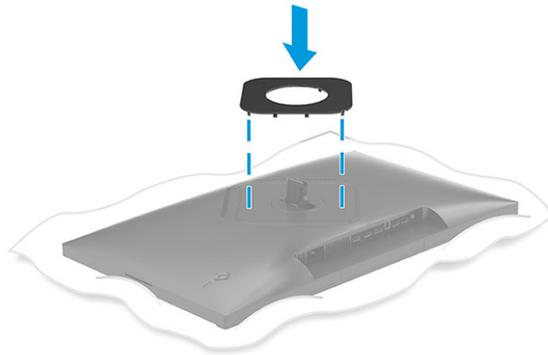
2. Align the stand with the base (1), secure the latch (2), and tighten the screw (3).
