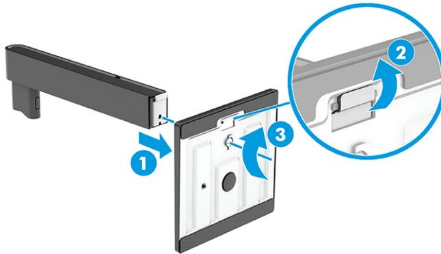
3. Attach the stand to the back of the monitor.
