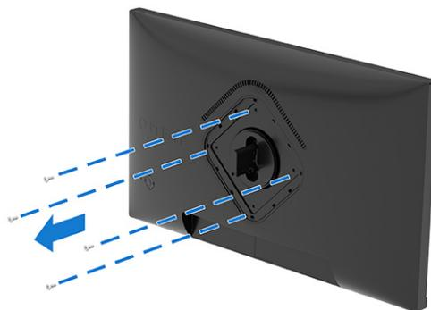
2. Remove the hinge from the VESA recess located on the rear of the monitor head.
