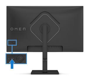
Press the power button on the monitor to turn it on.
