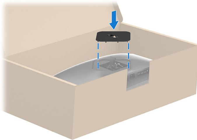
2. Align the base with the stand (1), secure the latch (2), and tighten the screw (3).
